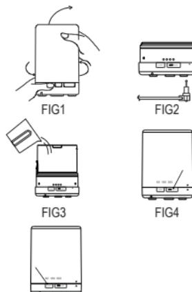
Use the graduated container to fill the water tank. Fig3
